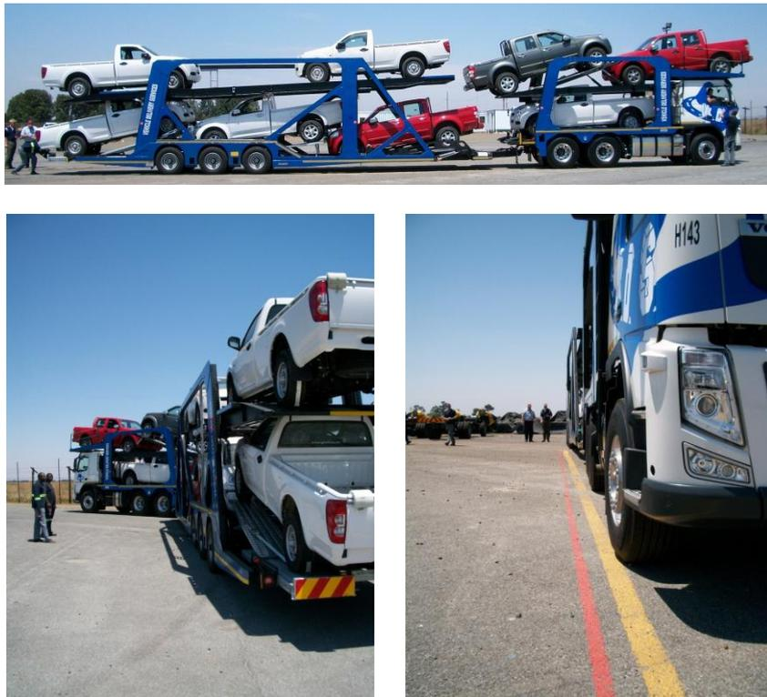
**Figure 3: The modified Unipower Maxiporter undergoing low-speed turn testing**
