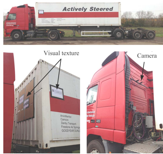
Fig. 7. The test vehicle, showing the location of the camera and the arbitrary visual texture added to the trailer.
