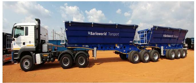
Fig. 5b 21.6 m, 73.7 t B-double side-tipper
