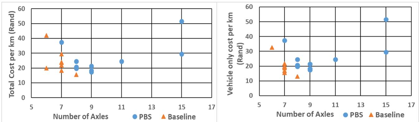
Figure 1: Total operating costs (left) and total vehicle only operating costs (right)
